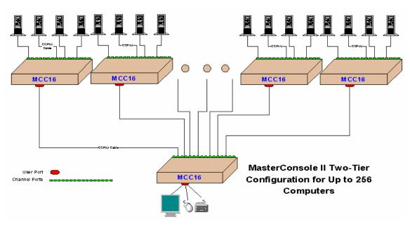
Figure 32 Two-Tier Configuration of up to 256 Computers
